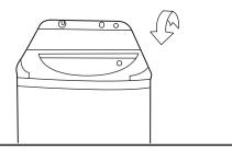
If you open the top lid, the machine will stop working before spinning.
